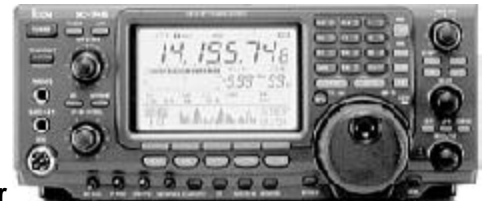
IC-746PRO HF, 6m, 2m All mode w/ DSP and auto tuner
