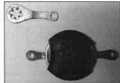
Figure 4 — A pair of toothed-washer solder lugs are held tightly in place against a button-cell battery to make a replacement battery for the Kenwood TS-940 (and probably many other radios).
